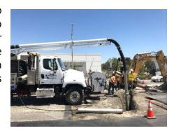
**2-Recycle Combination Trucks** Manufactured by Bucher. These trucks use 90% recycled water from the collection system to clean the pipes.
