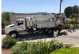
**1 -Specialty Easement Cleaning truck with 1200' of cleaning capability-** Sewer cleaning hose capability of 1200'/80 GPM/1" diameter hose/2000psi. It is ideal for easement type cleaning and difficult to reach areas.
