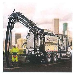
The KAISER PREMIER AquaStar offers a perfect combination of performance and versatility. The KDU jetting pump delivers water at a rate up to 132 gpm and water pressure of up to 2900 psi. The large hose reel can accommodate up to a
